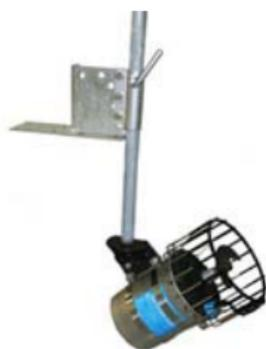
The de-icer unit may be extended down from the surface mounting bracket to a maximum length of 10 feet. Due to shipping limitations, users must supply their own 1" O.D. pipe extensions.
