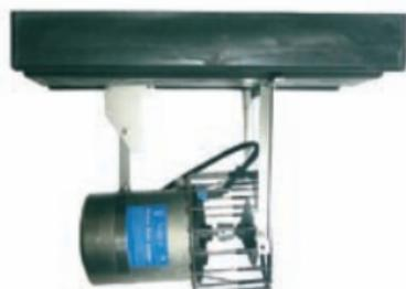
The De-icer unit is mounted at an angle just below the flotation block. Angle operation of de-icer produces an elongated pattern of agitated water and is well-suited for shallow water operation. All models can be used with this float.
